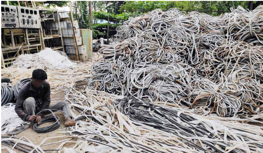
A worker is separating the plastic cover of recovered wires from dismantled ships.
